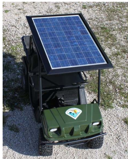
Figure 3: Electric Vehicle showing an example of a solar roof installed.
